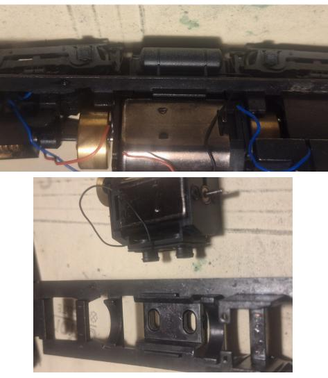
STEP 3: Remove fly wheels by prying gently with a flat bladed screwdriver.
