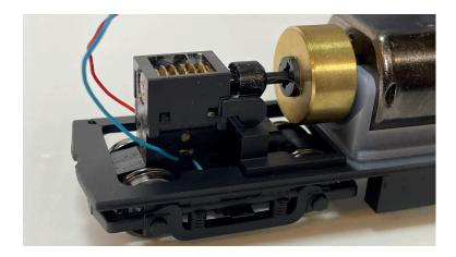
STEP 17: If you have opted for the powered rear truck, install it in a similar Manner. Painting the driveshaft black is recommended. The position of the rear Flywheel can be adjusted to allow proper flex in the rear truck while maintaining Shaft engagement. Solder the pickup wires to the motor or install a decoder.
