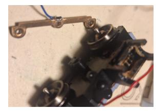
STEP 14: If building with one powered truck use the Wheel Chuffs, Wheels, and Rear Truck to assemble the rear trucks.
