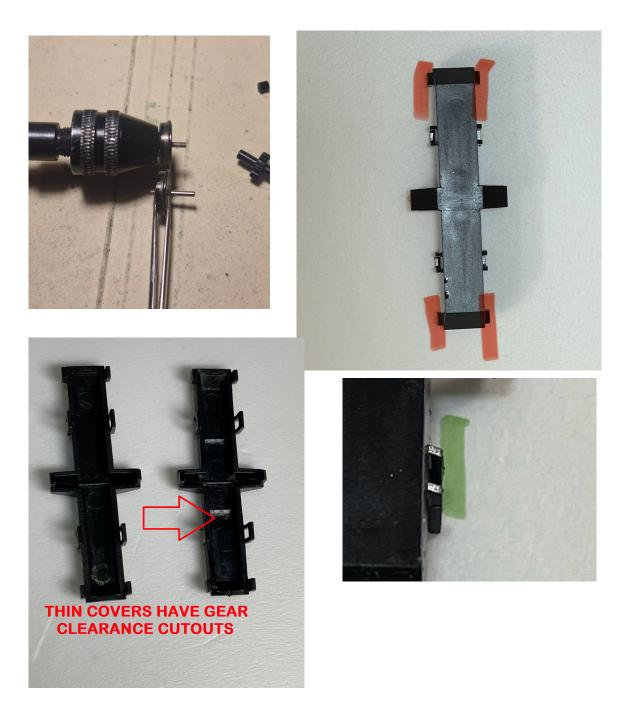
STEP 11: Cut the extensions from the gear tower flush with the wall. Keeping the blade angle towards the outside helps keep this cut straight.
