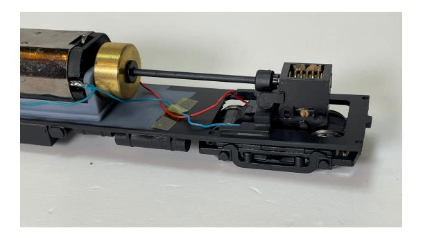
STEP 18: Carefully remove the two red highlighted 3D printed braces in the photo. The four black areas are used to mount the floor to the shell.
