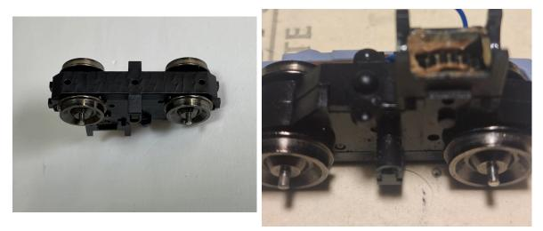
STEP 13: Replace power pickups and new side frames "L". Pop black wire keepers from power pickup and cut tab flush, proceed to solder wires to each pickup.
