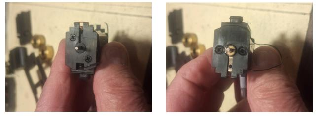
STEP 5: Remove motor cradle from motor.
