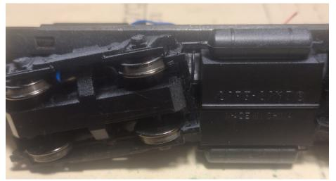
STEP 2: Remove trucks and motor by removing screws that hold weight to frame. Then remove the motor from the frame.
