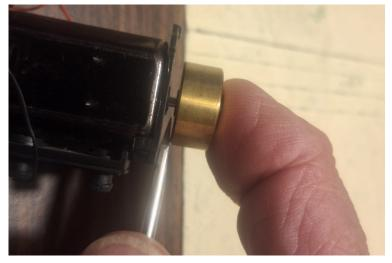
STEP 4: Remove motor cradle screws, two at each end of motor, and set aside.
