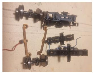
STEP 8: Remove wheel and axle halves from center gear. Place center gear in cutoff jig. Cut the ends of the center gear that extend outside the jig will give the correct HOn3 spacing.
