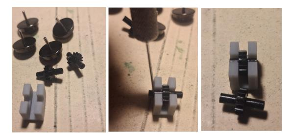
STEP 9: Place wheel in the axle cutting Jig. Using a cutoff disc, cut along the edge of the jig. Don't worry about damaging the jig, you will throw it away. It is more important that the axle is cut flush. Axles that are too long can touch in the gear chuff and cause a short. Repeat for all eight wheels.
