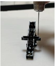
STEP 12: Insert the wheels into the tower and gently snap the gear cover back into place. Be sure everything is correctly done before this step, the gear cover cannot be removed without pulling the wheels off.
