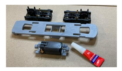
STEP 15: Install the hex couplers into the worm drive, then install the trucks, ensuring the worm cover is snapped onto all four bosses. Check for proper truck flex.
