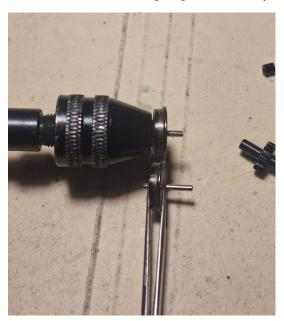
STEP 11: Cut the extensions from the gear tower flush with the wall. Trim excess with a hobby knife.
