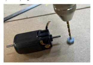
STEP 5: Press hex nuts onto motor shaft until flush or nearly flush.
