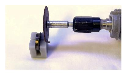
STEP 10: When cutting is complete clean up the end of the axles with a file or sandpaper. Chucking the axle into a motor tool or small drill at low speed can speed up this process. Reassemble the axles into the gear muffs. Use a HOn3 flange gauge to check that the axles are gauged correctly.
