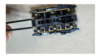
STEP 8: Remove wheel and axle halves from center gear. Place center gear in cutoff jig. Cut the ends of the center gear that extend outside the jig will give the correct HOn3 spacing. Be sure to cut flush, use a sharp chisel blade.
