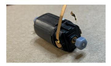
STEP 6: Insert motor into 3D printed cradle, centering it in the frame. Cradles are marked L for the end with the wires and S for the blank end. Once everything is lined up secure with superglue.
