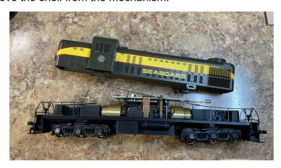
STEP 2: Remove handrails and motor by removing four screws from the bottom of the locomotive. Then cut the power tabs that hold the motor to the circuit board. Finally CAREFULLY remove the covers from the worm gears, releasing the trucks. This is best done by reaching up between the wheels.
