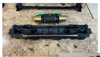
STEP 3: Remove fly wheels by any means necessary. Good luck. Sometimes they come off, sometimes they don't. Cut 1/8" (0.125") off each shaft and sand or file ends smooth.
