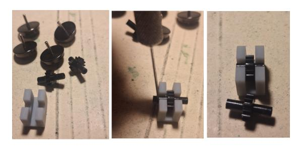
STEP 9: Place wheel in the axle cutting Jig. Using a cutoff disc, cut along the edge of the jig. Don't worry about damaging the jig, you will throw it away. It is more important that the axle is cut flush. Axles that are too long can touch in the gear chuff and cause a short. Repeat for all eight wheels.
