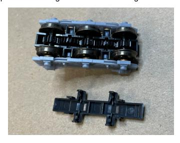
STEP 13: Double-check the wheel gauge, the tabs will often push the wheels out.
